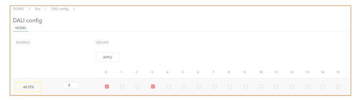
As confirmation of the assignment of the address to the group, the box changes from red to blue
