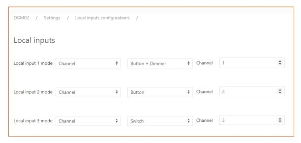
The image above shows the possible settings, from web server, of the Local Inputs as "Channel". By setting the local input in "Channel" it is possible to control only one physical channel of the 512 available.
