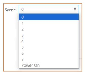
By setting the local input as "Scene", it is possible set up to 8 scene, from 0 to 7, or by configuring the "Power On" scene, it is possible to define the values of the 512 channels when the DGM02 is turned on.
