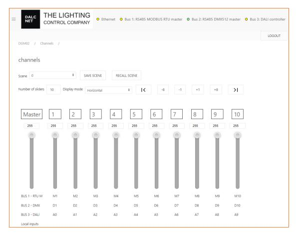
The DGM02 has a WebApp for the supervision and regulation of all the channels available in the various DALI, DMX, MODBUS protocols, which can be used from any device equipped with a compatible browser.
